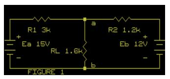
Step 1 E<sub>a</sub> is present, E<sub>b</sub> is removed. Refer to figure 2. Remove E<sub>b</sub>, and replace it with a short. (This assume that the voltage source has no internal resistance.) Solve for the magnitude and direction of the current through R<sub>L</sub> in figure 2. Calculate the voltage drop across R<sub>L</sub>. Determine the polarity of the voltage drop. Record the current, its direction, the voltage drop and the polarity on figure 2. Show your calculations in space provided.
